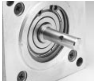
Cross-drilled shaft accepts hardened roll pin to attach sleeves, pulleys and gears.
