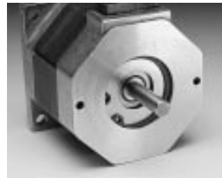
Encoder-ready rear shaft extension and mounting provision (1.812" Bolt circle) accepts popular encoders.
