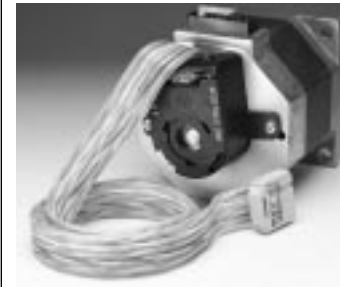
HP HEDS 5600 encoder with line driver outputs and preterminated ribbon cable.
